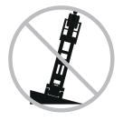
If the tilt alarm sounds: Lower the platform. Move the machine to a firm, level surface. If the tilt alarm sounds when the platform is raised, use extreme caution to lower the platform.
